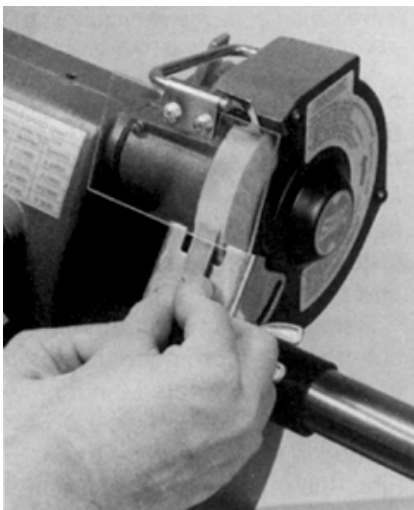
Figure 24-33. If the chisel is narrower than the width of the wheel, hold the chisel there momentarily, then back it away.
