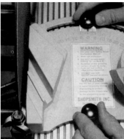
Figure 24-43. Position the cutter fully in front of the disc and lock the guide in place.
