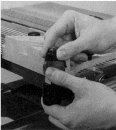
Figure 24-42. Hold the cutter wing against the sharpening guide and tighten the nut finger tight.
